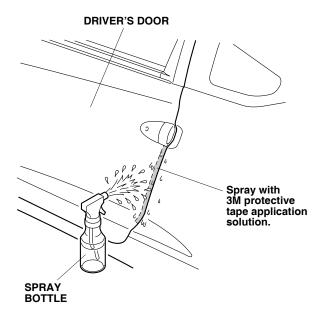
Open the driver's door. Peel back about 50 mm of the adhesive backing from the left door edge film. Align the v-notch on the left door edge film to the driver's door as shown.
